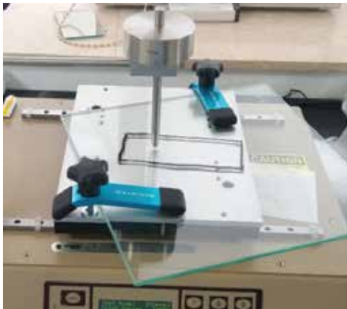
The drill rubbing the glass sample for appox 10,000 times.
